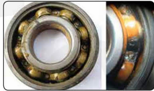
Typical Standard Ball Bearing Seal (32 hours)
